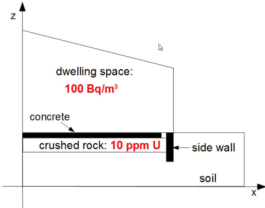
**Figure 1.** Modelling the contribution of a drainage layer to indoor radon concentrations, after Watson et al. (2013) and Andersen (2000).
