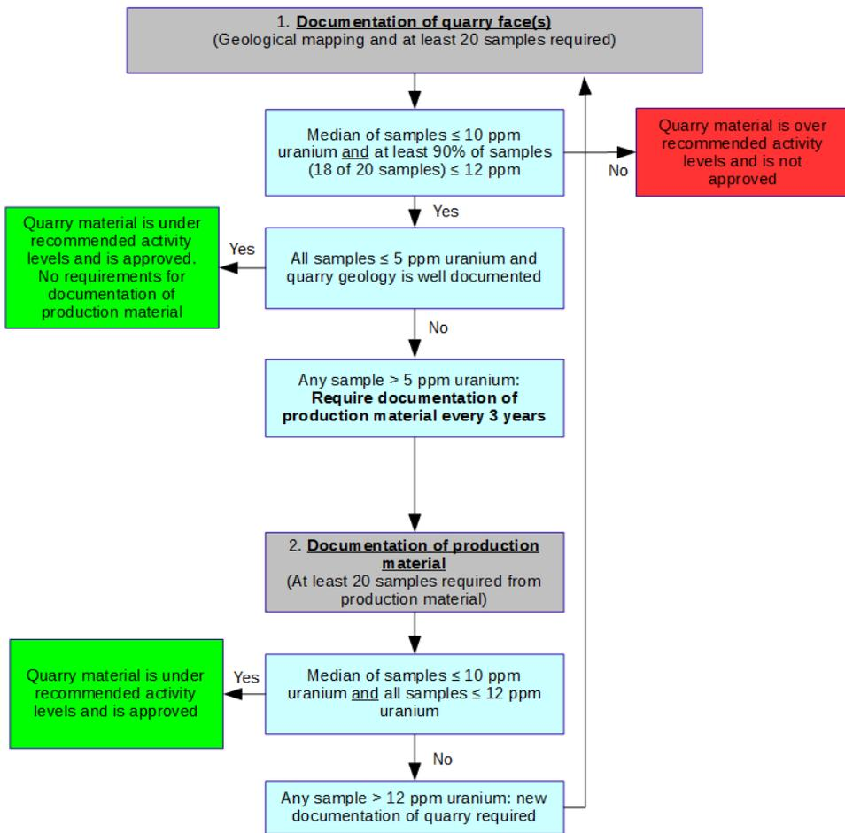
Figure 2. A sampling methodology for quarry material.
