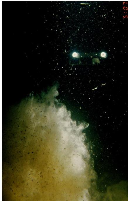
**Figure 2.** Floc Camera Assembly in-situ image of flocs in seawater (from image library of JPM Syvitski collected in Goose Bay, Labrador). The image shows a resuspension plume stirred up from the floc camera hitting the seafloor (bottom left). Above and to the right is the ambient background seawater containing flocs settling.
