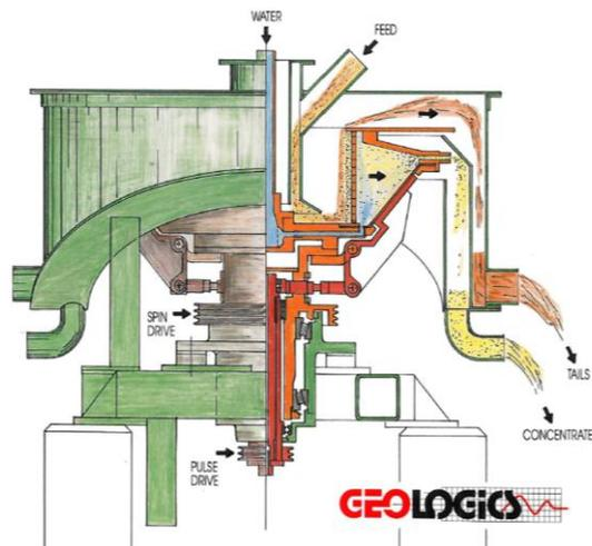
**Figure 3.** Kelsey Jig J200 (left) and principle of operation (right).
