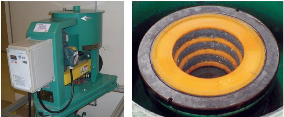
**Figure 2.** Knelson Concentrator (left) and inside concentrating cone with sediment layer (right).
