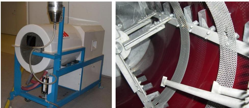
**Figure 1.** Mozley C900 MGS (left) and inside drum scraper assembly and feed system (right).
