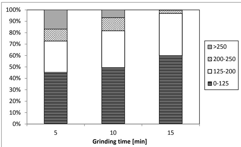
**Figure 2.** Contents of fine size fractions in HPGR product for  $F_{sp} = 2\text{N/mm}^2$ .
