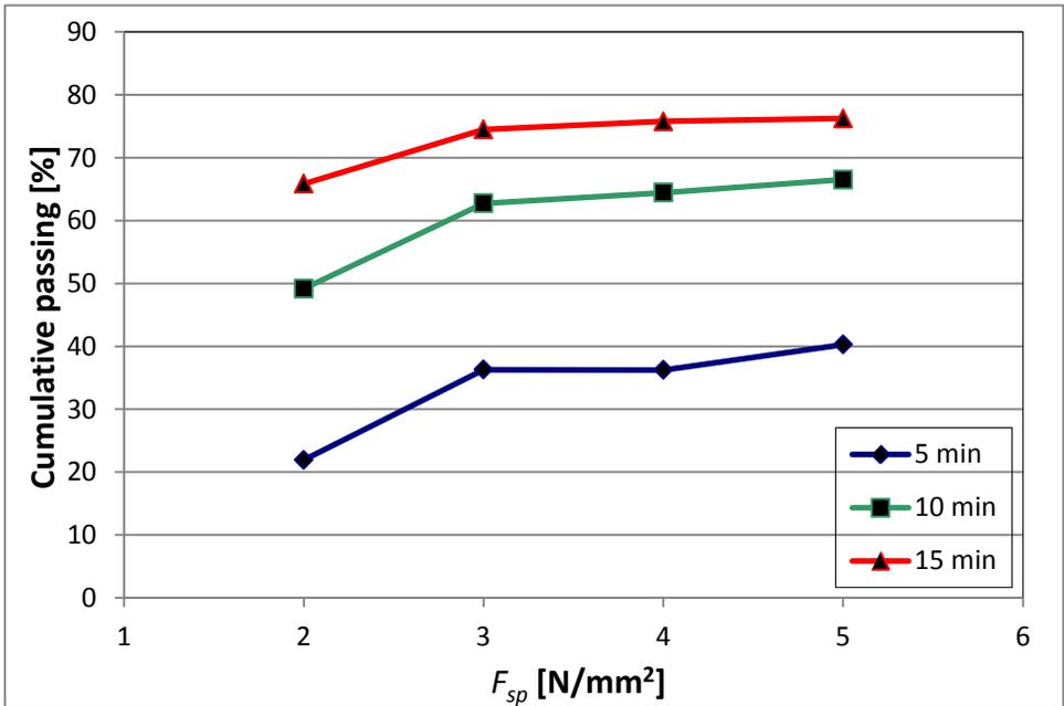
Figure 6. Relationship between the  $F_{sp}$  and the -0.125 mm size fraction recovery at different grinding time.
