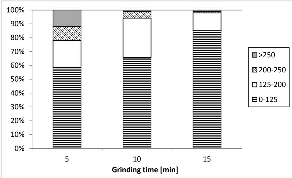
Figure 3. Contents of fine size fractions in HPGR product for  $F_{sp} = 3\text{N/mm}^2$ .
