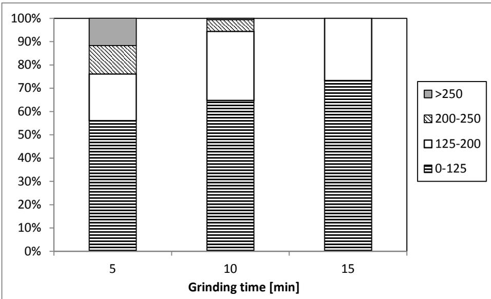
Figure 4. Contents of fine size fractions in HPGR product for  $F_{sp} = 4\text{N/mm}^2$ .
