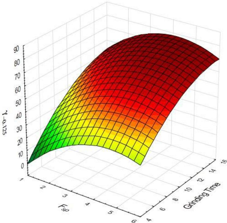
**Figur 7.** Recovery of -0.125 mm size fraction as a function of grinding time and  $F_{sp}$
