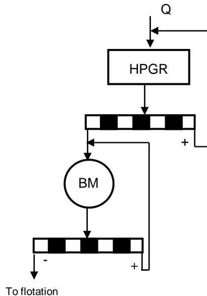
**Figure 1.** Typical combination of HPGR and ball mill in ore comminution circuit
