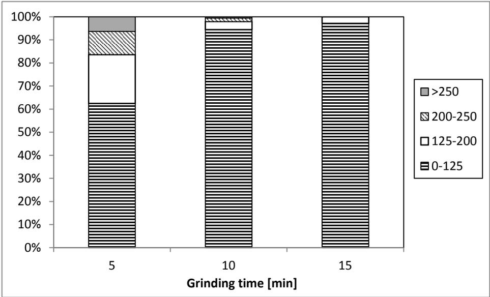
Figure 5. Contents of fine size fractions in HPGR product for  $F_{sp} = 5\text{N/mm}^2$ .
