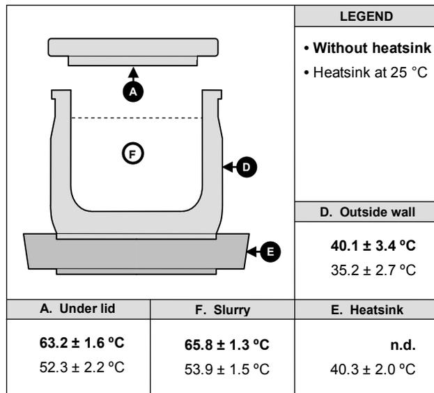
**Figure 3.** Average measured surface temperature (±1 SD) after 30 min of wet grinding.
