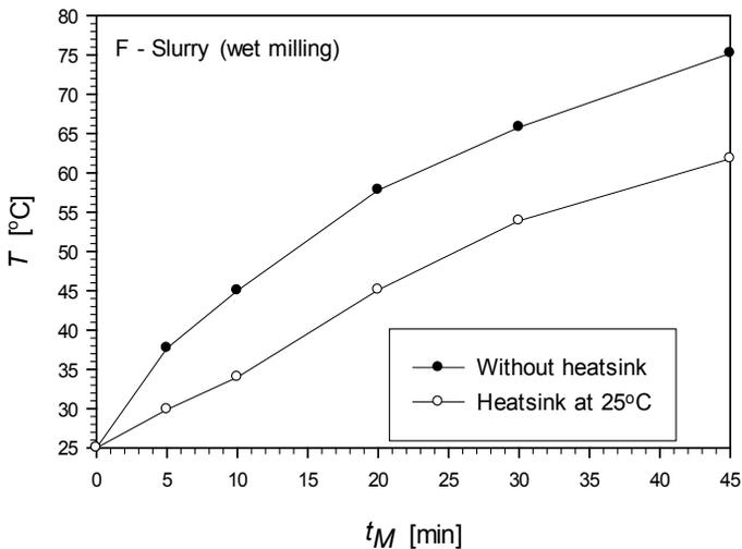
**Figure 5.** Temperature in the slurry as a function of grinding time.
