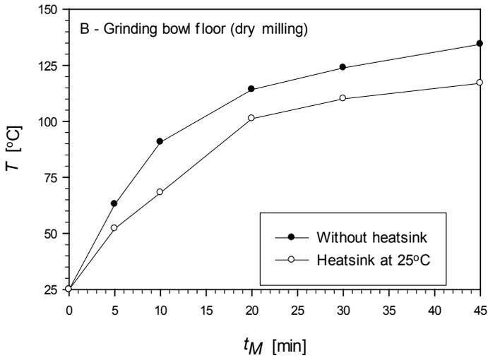
**Figure 4.** Surface temperature at the grinding bowl floor as a function of grinding time.
