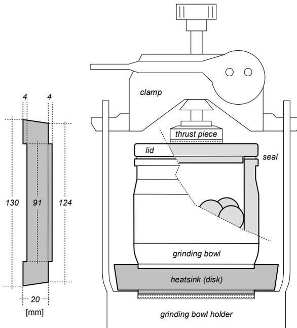
**Figure 1.** The heatsink, grinding bowl and grinding bowl holder.
