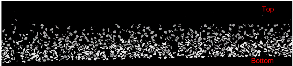
Figure 2. BSE image of vertical cut polished section. Silicate (gray) and iron sulfide (white) concentrate (104-147 \mu\text{m} ) mixed with fine graphite, sample:graphite 1:1 weight ratio. Segregation is evident as the heavy particles are concentrated towards the bottom.
